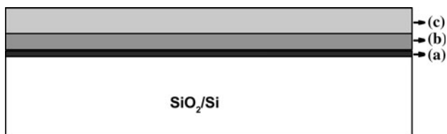
Fig. 1 PZT/ \text{IrO}_2 / \text{TiO}_2 / \text{Ti} / \text{SiO}_2 / \text{Si} structure. (a) (3 nm) \text{TiO}_2 /(10 nm) Ti seeding layers, (b) (200 nm) \text{IrO}_2 layer, and (c) (200 nm) PZT layer
